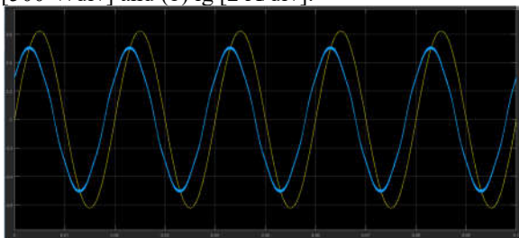
Fig. 15. Experimental results of the proposed topology with leading power factor operation. (a) v_g [500 V/div] and (b) i_g [2 A/div].
