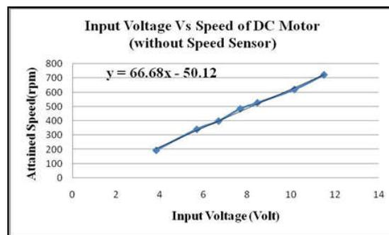
Fig.4. Open Loop Speed Variation withappliedvoltage without SpeedSensor
