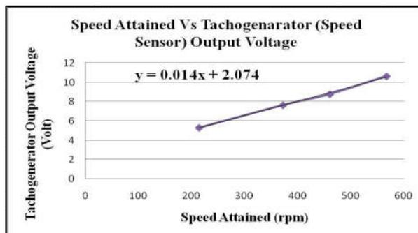
Fig.7.VariationTachogenerator Output Voltage with Speed Attained by DC Motor
