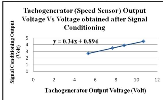
**Fig.8. Variation of Signal conditioning output with Tachogenerator Output Voltage**
