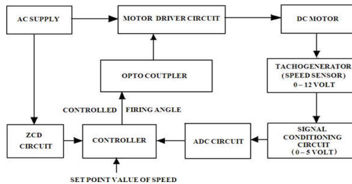
**Fig.1. Block Diagram of Closed Loop DC Motor Speed Control System**
