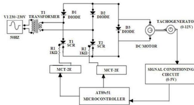
**Fig.3. Interfacing between 8051 microcontroller and DC Motor Driver Circuit**
