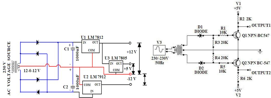
**Fig.2.Circuit Diagram for Power supplydesigned**
