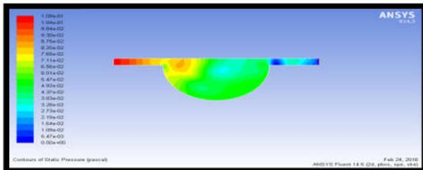
According to the pressure plot the maximum pressure value  $1.09e-01$  Pa and minimum pressure value  $5.47e-03$ . The maximum pressure at inlet condition of combustion chamber and minimum pressure value at outlet conditions of the combustion chamber.
