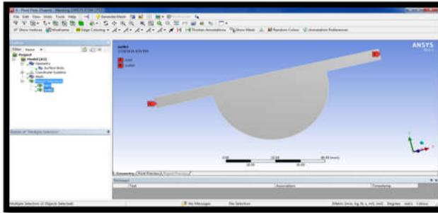
Boundary conditions are a required component of the mathematical model. Boundaries direct motion of flow. Specify fluxes into the computational domain, e.g. mass, momentum, and energy. Fluid and solid regions are represented by cell zones. Material and source terms are assigned to cell zones. Boundaries and internal surfaces are represented by face zones. Boundary data are assigned to face zones.
