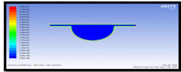
According to the Heat transfer coefficient plot the maximum velocity value  $6.00e+01$  w/m<sup>2</sup>-k and minimum Heat transfer coefficient value  $3.00e+00$  w/m<sup>2</sup>-k. The maximum Heat transfer coefficient at complete boundary of combustion chamber and minimum Heat transfer coefficient value at inside of the combustion chamber.
