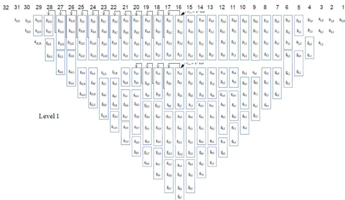
Fig.5. Architecture for level 1 of 16-bit Multiplier B
