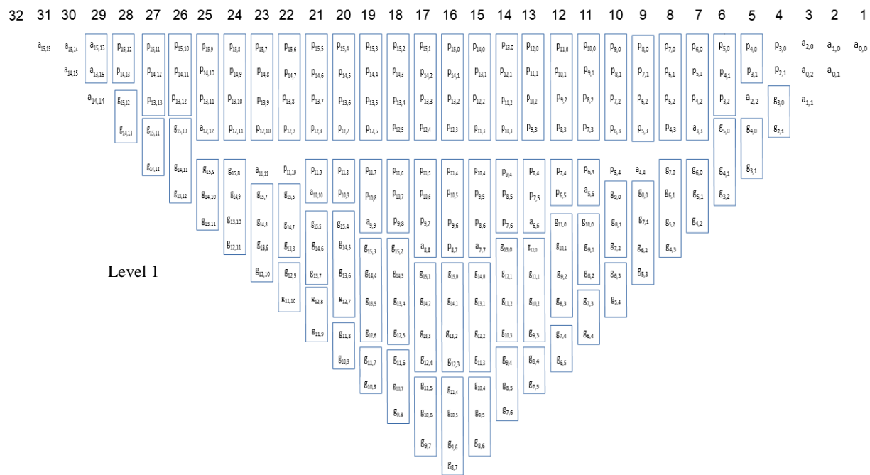
Fig.3. Architecture for level 1 of 16-bit Multiplier A
