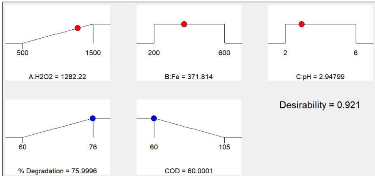
Fig 5.1: Results of optimization for Photofenton treatment
