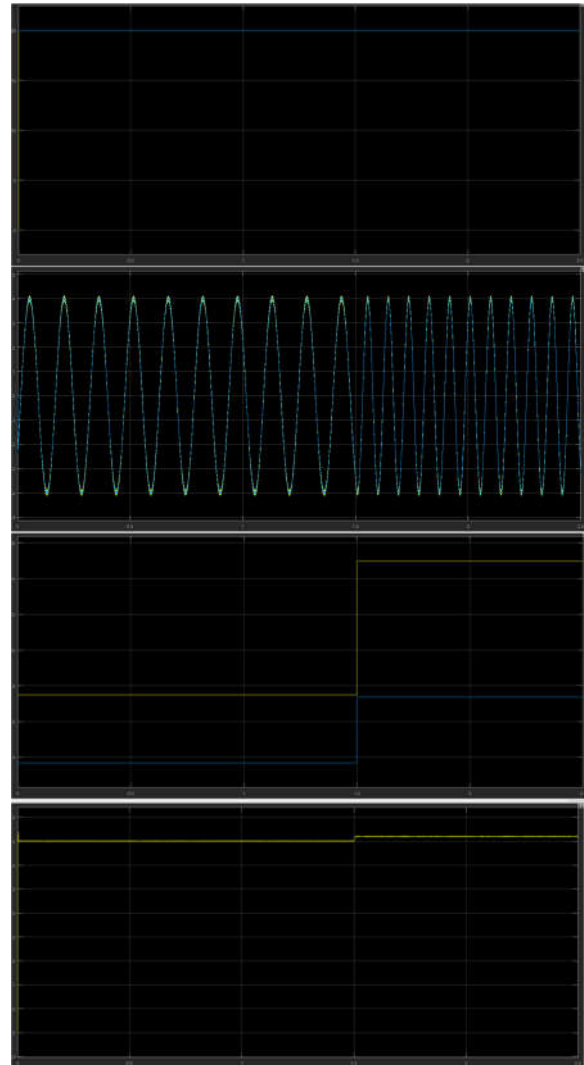
Fig. 12. Simulated speed, stator currents, and quadrature current responses of an FSTP inverter-fed IM drive for a sudden increase in stator and rotor resistances at a speed reference 20 r/min using (a) proposed ANN.
