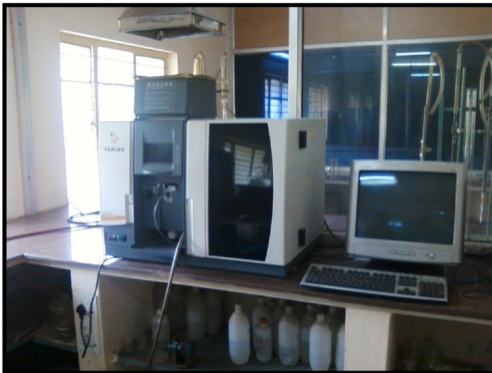
Figure-3 Fast Sequential Atomic Absorption Spectrometer
