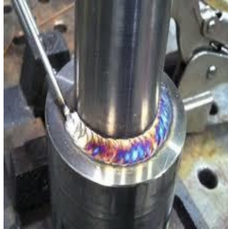
TIG welding surface look
