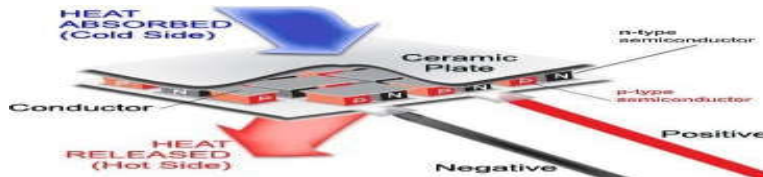
Figure 6.1 Operation of TEC
