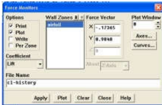
Fig. 34. Force Monitors window set to monitor the lift coefficient for an angle of attack of 10^\circ .
