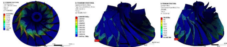
Fig 5 (a) Total Deformation (b)Equivalent Elastic Strain (c) Equivalent stress
