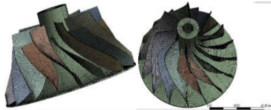
Fig 4 meshing of impeller
