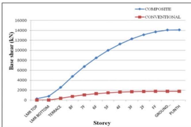
**Fig:** Comparison of composite and conventional (RC) building for base shear
