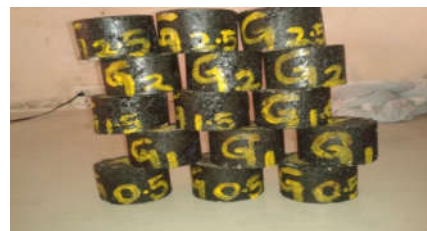
Marshall Moulds Using Glass Fibres
