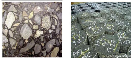
Dense graded HMA surface Dense-Graded Core sample
