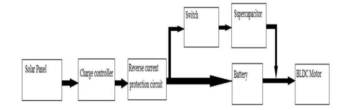
This is the design of the integration of battery and super capacitor for electric vehicle by connecting them in parallel to each other. This integration of storage devices will overcome the disadvantages of each one and increase overall performance of storage unit.
