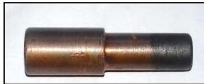
Figure 6. Copper Electrode after Machining
