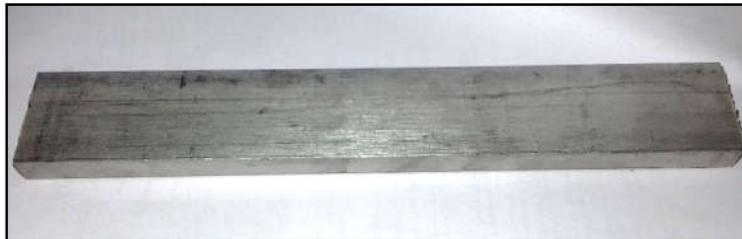
**Figure 3. SS-316L as a Work piece material-130 mm×40 mm×12 mm**
