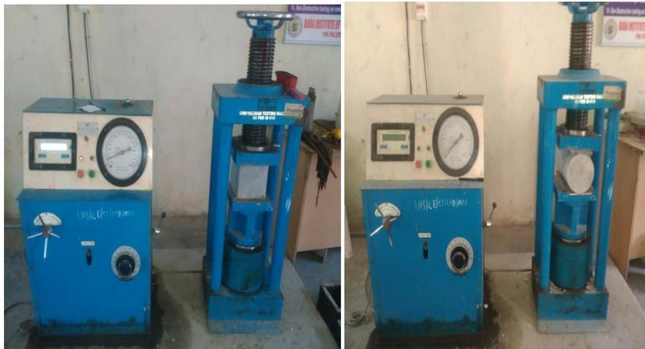
Fig.2 Compressive strength test & Tensile strength test
