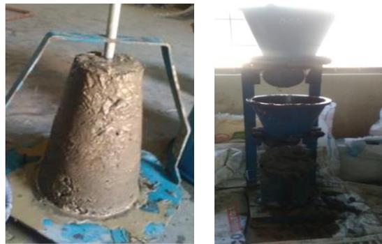
Fig1 Slump Cone test & Compacting factor test
