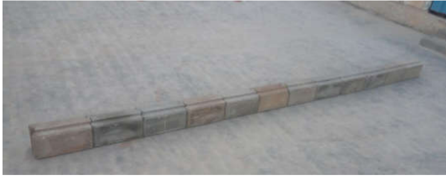
Fig 4: Dimensional test of Interlocking Blocks
