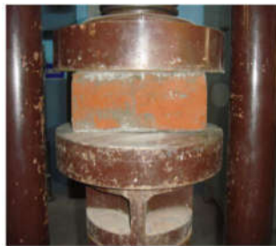
Fig 3: Compression test setup of normal brick
