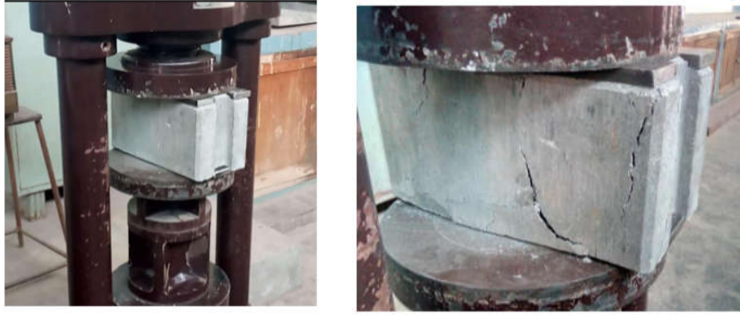
Fig 2: Compression test setup of Interlocking and Compression test setup of Interlocking Block
