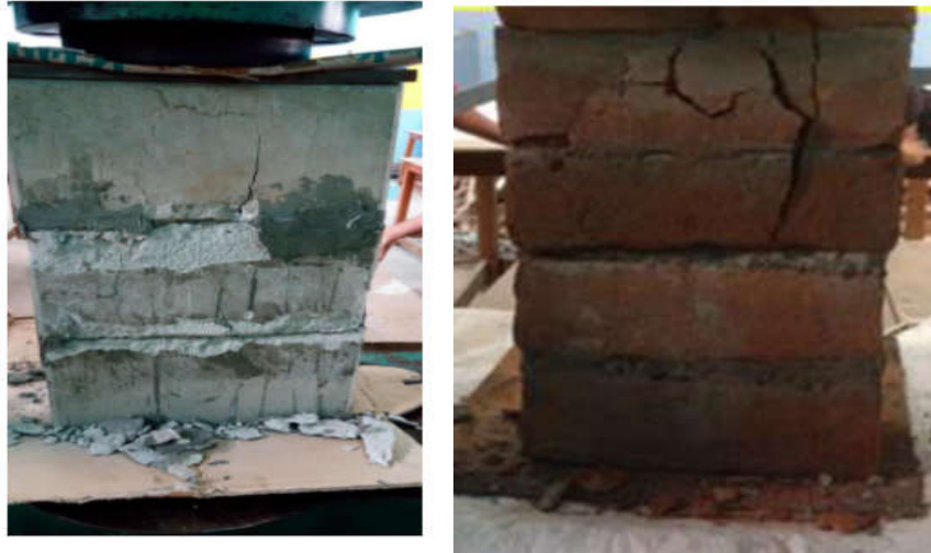
Fig 6: Failure mode of interlocking and normal brick
