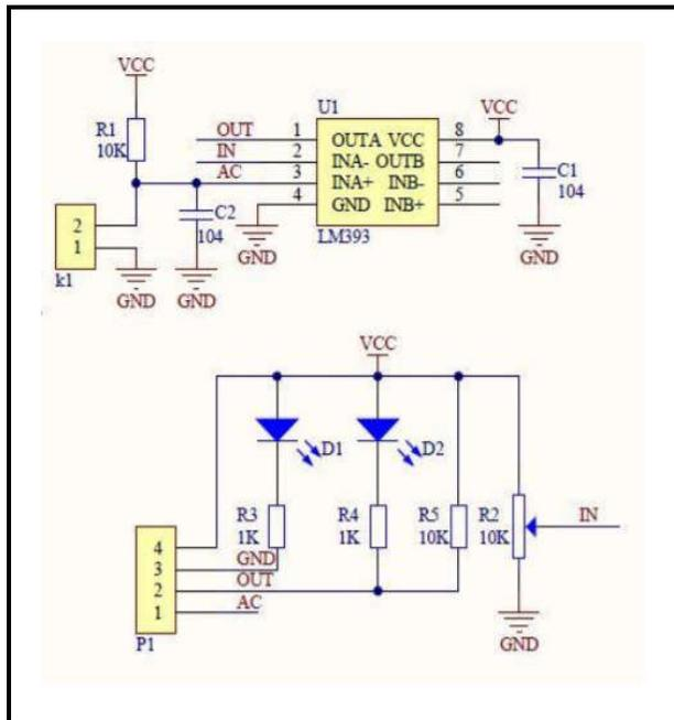
Fig 6. Schematic Diagram of Rain Sensor
