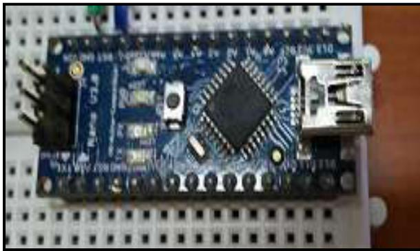
Fig 3. Arduino Microcontroller
