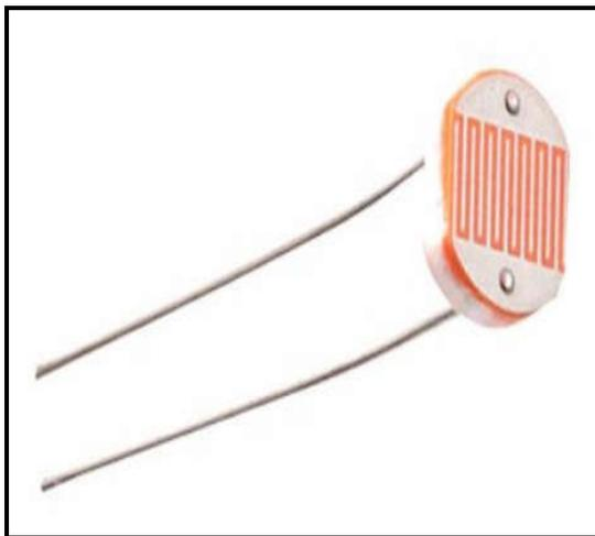
Fig 4. Light Dependent Resistor
