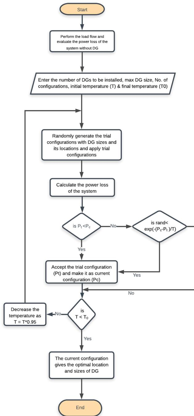
Figure 2: Flowchart of Process Using Simulated Annealing Algorithm
