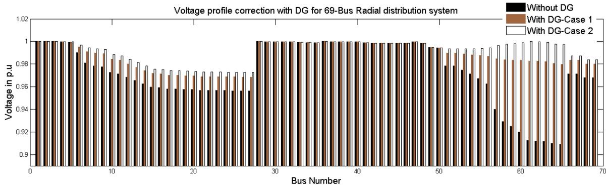
Figure 8: Voltage profile correction with DG for 69-Bus Radial distribution system
