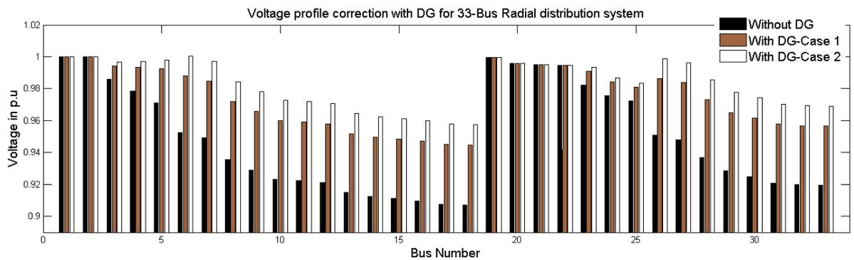
. Figure 3: Voltage profile correction with DG for 33-Bus Radial distribution system
