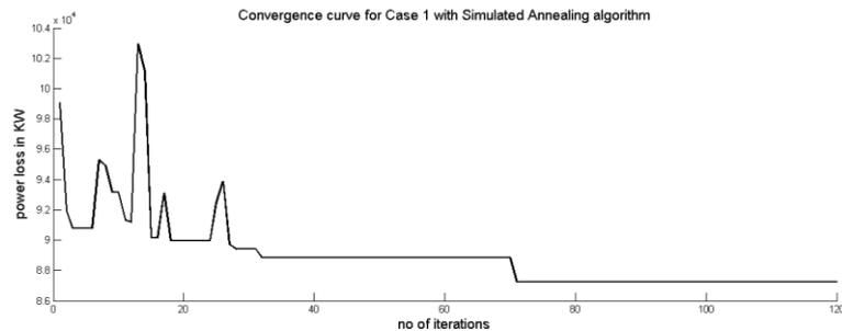
Figure 4: Convergence curve with SA algorithm for test case 1
