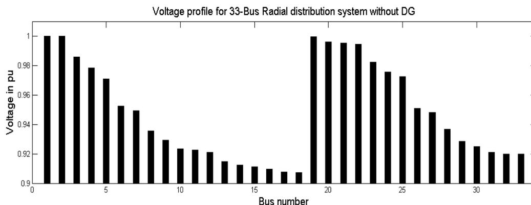
Figure 1: Voltage Profile For 33-Bus Radial Distribution System Without DG
