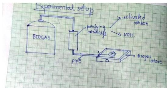
The KOH will absorb the CO<sub>2</sub> content that is present into the biogas. Passes out the rest component or gases throughout the pipe. The reaction is shown below.
