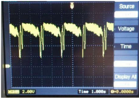
Figure 10: Voltage measurement from a Sensirion SLQ-HC60 flow meter connected to the peristaltic pump.
