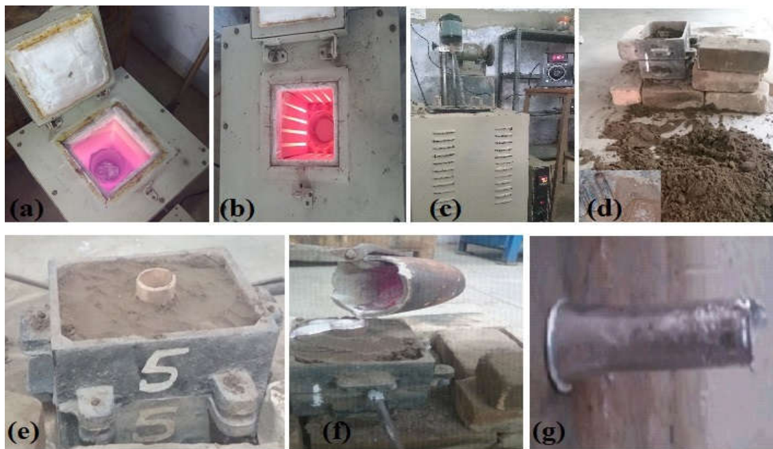
Fig. 2 MMC fabrication using pit (a) melting of aluminium (b) adding of reinforcement \text{Al}_2\text{O}_3 particulates (c) manual stirring through steel rod (d) prepared mould (e) pouring of molten material (f) solidification of molten material (g) dragging of solidified MMC (h) fabricated \text{Al}/\text{Al}_2\text{O}_3 MMC
