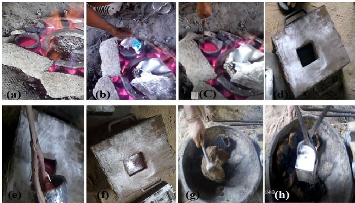
Fig. 1 MMC fabrication using pit furnace (a) melting of aluminium (b) adding of reinforcement \text{Al}_2\text{O}_3 particulates (c) manual stirring through steel rod (d) prepared mould (e) pouring of molten material (f) solidification of molten material (g) dragging of solidified MMC (h) fabricated \text{Al}/\text{Al}_2\text{O}_3 MMC
