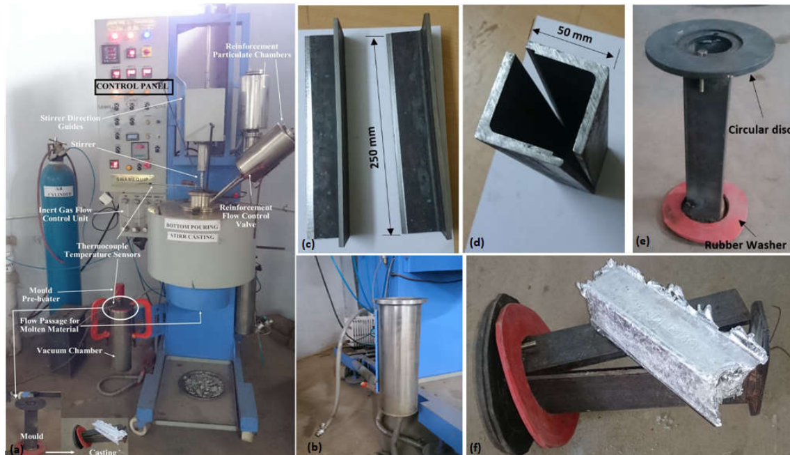
Fig. 3 MMC fabrication by BPSC(a)BPSC machine (b) vacuum chamber for mould (c) &(d) dimensions of the mould (e) prepared mould (f) fabricated Al/Al 2 O 3 MMC
