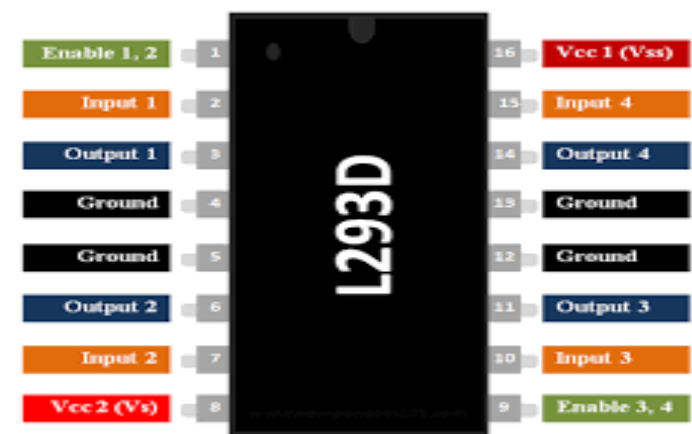
FIG: 2.7.2 PIN DIAGRAM OF IC L293D
