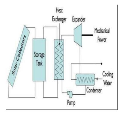
200°C. Both intensity of solar radiation as well as difference of temperature between entering fluid and ambient govern the efficiency of solar collector. The efficiency of such a system is lower than solar electric method using non-concentrating PV modules. Solar Mechanical is advantageous only when solar trackers are used but, the use of such systems is limited to large refrigeration systems only i.e. at least 1000 tons.
