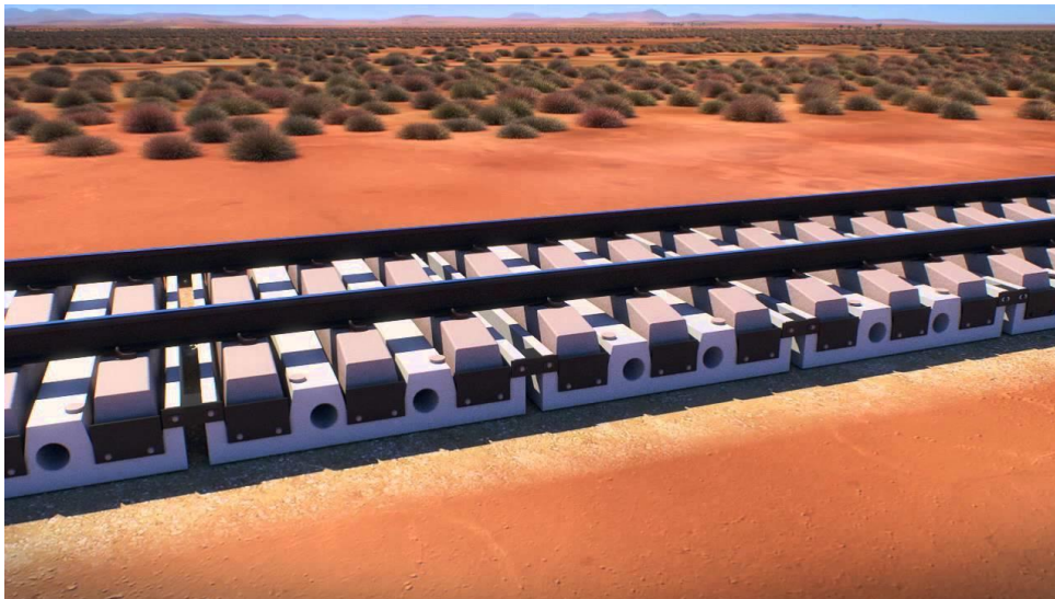
Figure 2. Sleepers with Casing Setup
