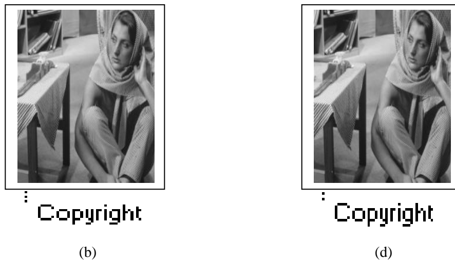
Fig 7 (a) Original Input Barbara Image for Watermarking (b) The Watermark Image (c) Invisible Watermarked Image (d) Watermark Recovered from Watermarked Image
