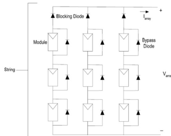
**Figure 3. Layout of a PV array**
