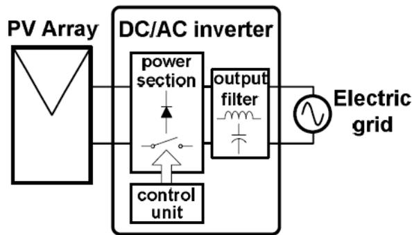
Figure 1. General Structure of Grid Connected PV Systems
