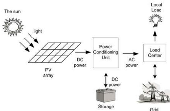
Figure 2. Main components of grid-connected photovoltaic systems
