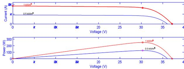
Figure 5. Matlab model I-V and P-V curves for various irradiation levels
