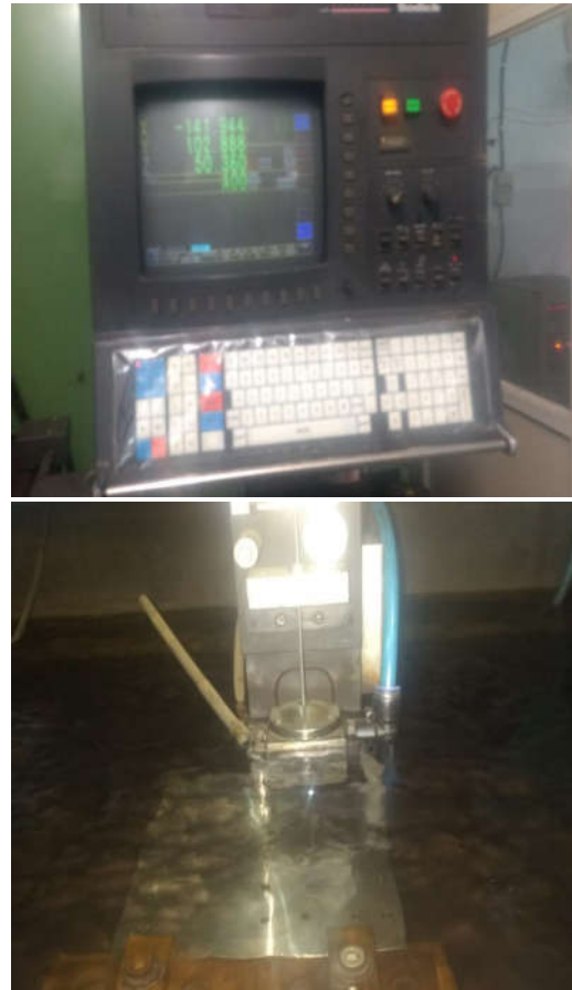
A) Setting the parameters for the machining B) Wire EDM processing of the material for roundness
