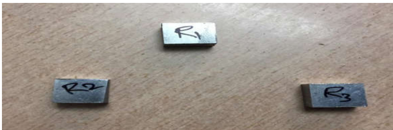
Fabricated test samples R1, R2, R3 for Radiography approach
