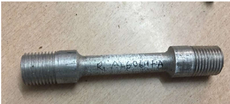
Tensile test sample R1 with mix of Al6061+Flyash
