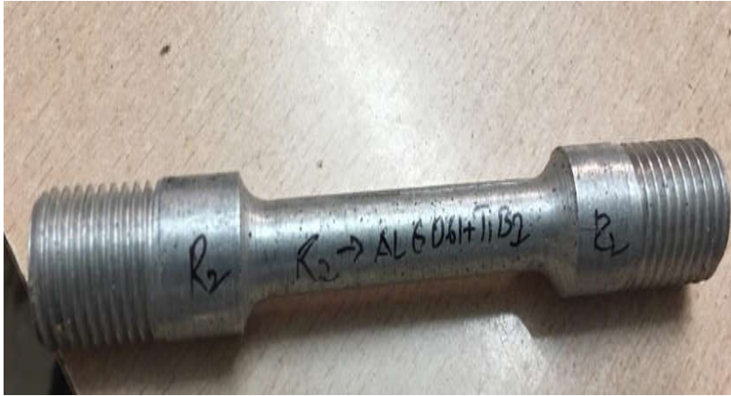
Tensile test sample R2 with mix of Al6061+TiB2
