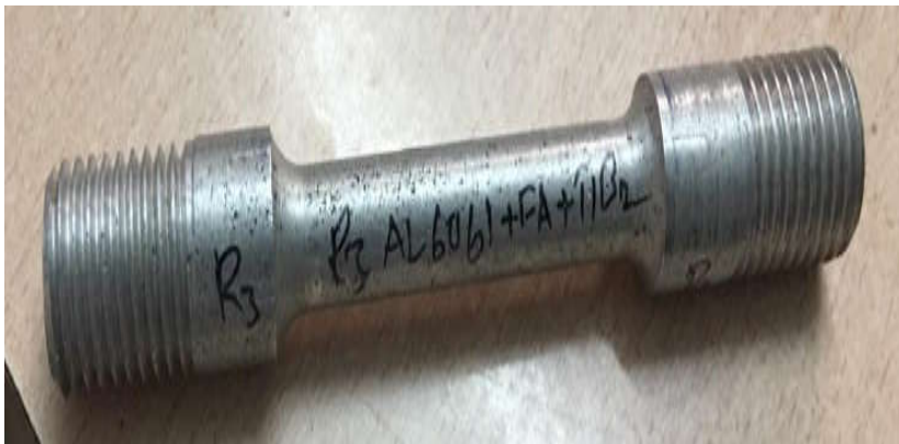
Tensile test sample R3 with mix of Al6061+TiB2+F.A
