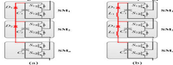
Fig. 3 Connection diagrams of SMs with balancing branches. (a) Using diodes to clamp capacitor voltages. (b) Using diodes and inductors to clamp capacitor voltages.
