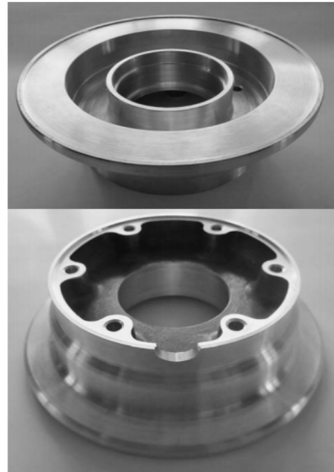
Figure 7: Finished product made from the forging by means of machining
