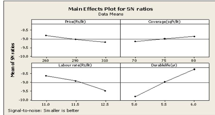
Figure 4. S/N ratio plots for various parameters of internal paint
