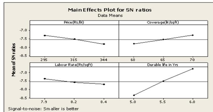
**Figure 3. S/N ratio plots for various parameters of external paint**
