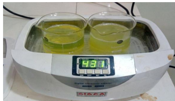
Fig 7. Mixture of CeO 2 & Bio Diesel Blends in Water Bath of Ultra Sonicator
