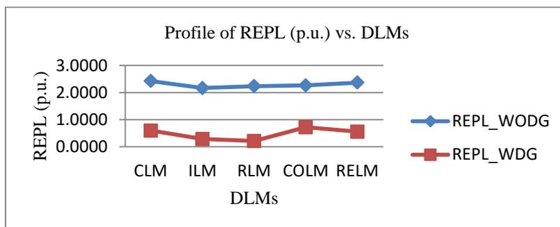
Fig. 24: Profile of REPL (p.u.) vs. DLMs
