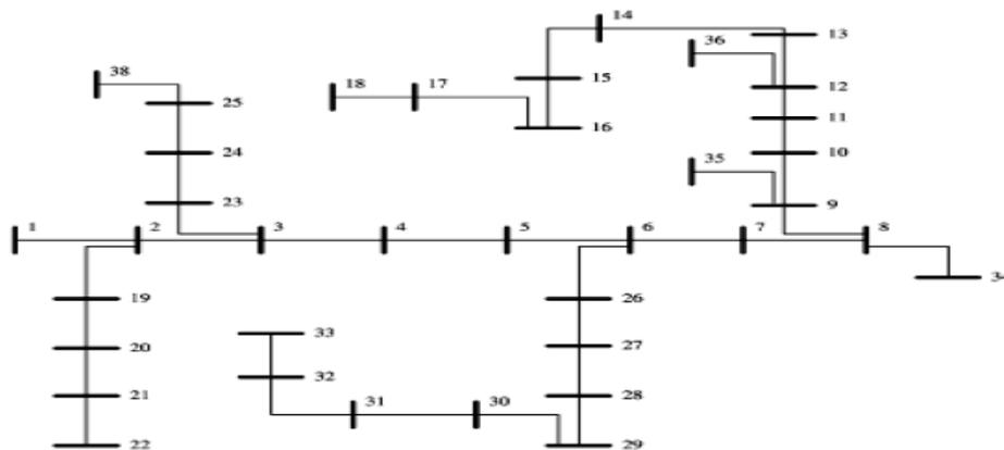
**Fig. 2:** Single line diagram of the IEEE-37 bus test system.
