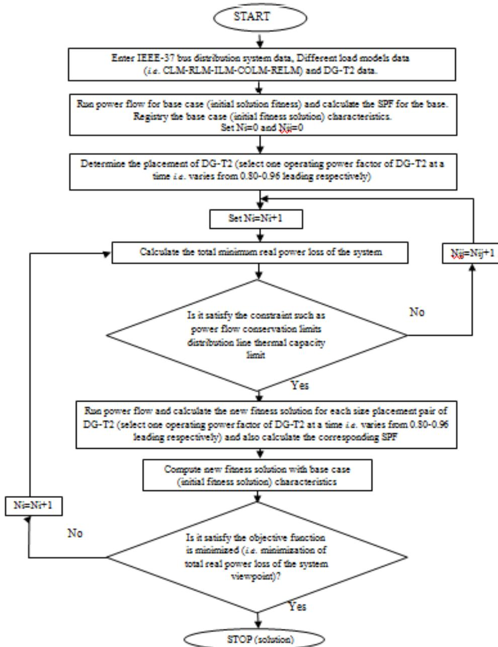
Fig. 1 : Schematic diagram of simulation programming
