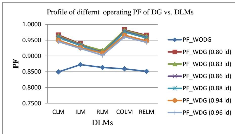
Fig 35: Comparison of different operating PF of DG vs. DLMs
