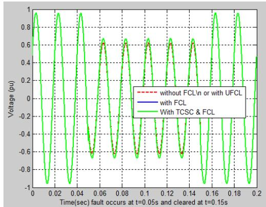
Fig.5: Voltage at bus MG3 during the fault at MG1.
