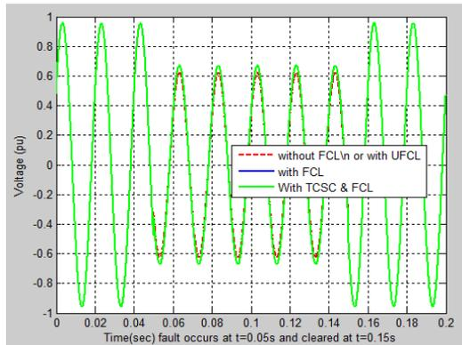
Fig.6: Voltage at bus MG3 during the fault at bus-49.
