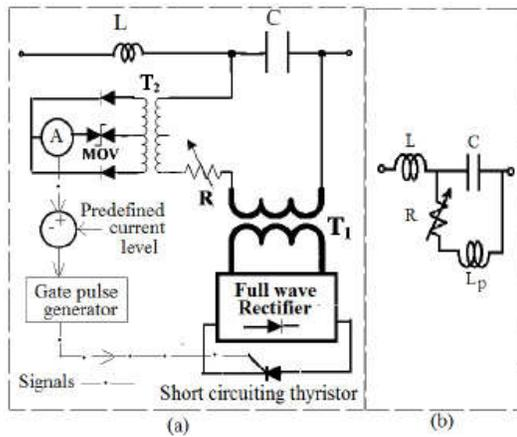
Fig.2: Resonant SSUFCL
