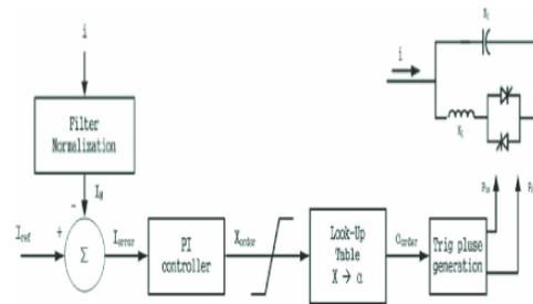
Fig.4: TCSC closed-loop constant current control methodology.
