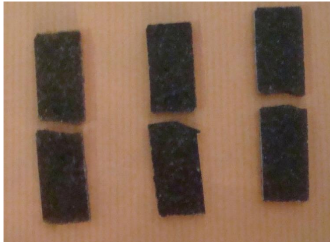
Figure 11 Almond shells filled polyester composite specimens after impact fracture
