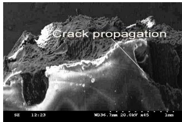
Figure 6. SEM Image of Impact tested C1 Composite
