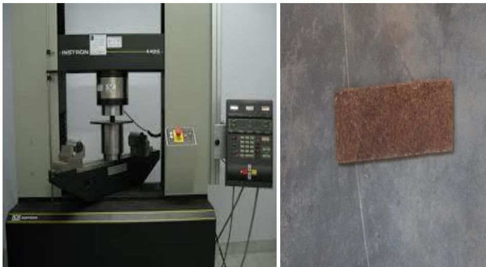
Figure 6 The Compression testing machine and particulate composite samples
