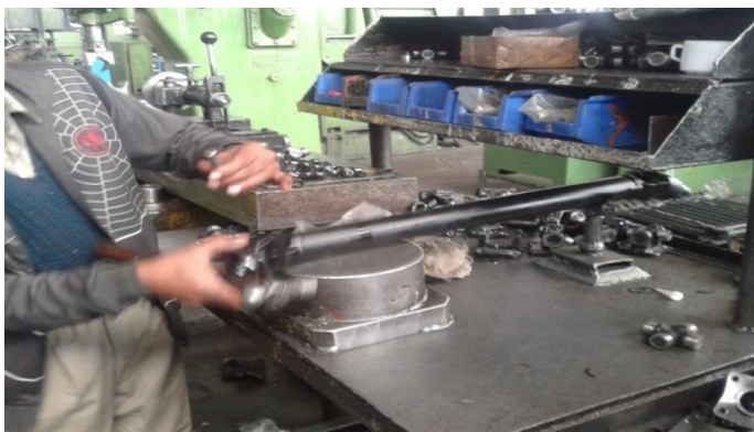
Fig 2: Rework being done on the painted shaft
