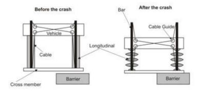
Thetelescope of whiteman conceptual design could also be conducted by fitting it behind the bumper, such that on an impact, the bumper-telescopic collapsible structure could absorb the impact, and through deformation of the longitudinal structure, absorb the kinetic energy involved to reduce the impact on the occupant of the vehicle. Its length is the only disadvantage in this proposed application, since the space behind the bumper is rather limited.
