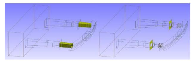
While collapsing the first supporting component of the support with the less inner dimensions comparing the second, slides incorporation with the folding front to the rear. After the complete change in shape all the folds would be packed in the first supporting component.
