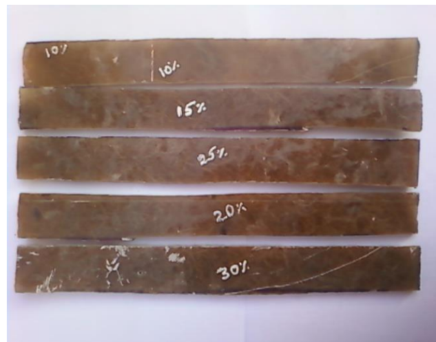
Figure 3 shows specimen (250mm × 25mm × 5mm) of 25 mm fiber length
