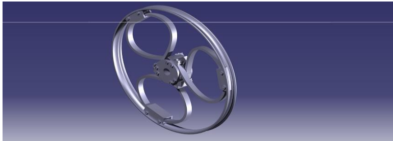
Fig 4.1 Catia model of loop wheel
