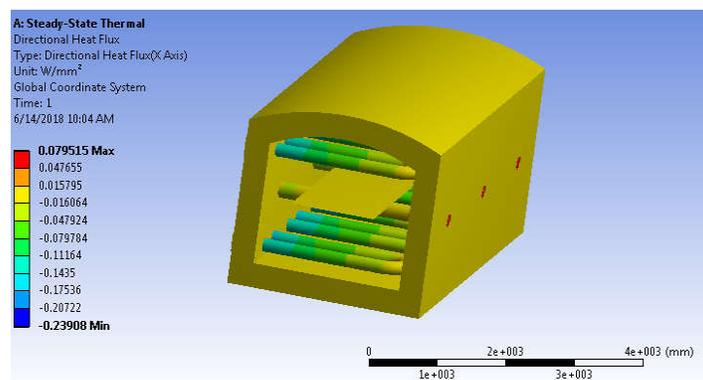
**FIG 3.5 DIRCTIONAL HEAT FLUX(here it shows heat transfer rate)**
