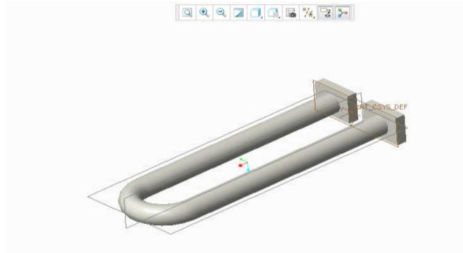
**FIG 1. 8 3D MODELS OF RADIANT TUBES**
