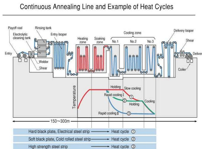
**FIG 1.1 CONTINUOUS ANNEALING FURNACE
