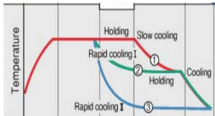
FIG 1.3 ANNEALING PROCESS(heating and cooling) TEMPERATURE VS TIME CURVE
