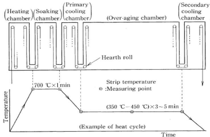
FIG 1.2 TEMPERATURE VS TIME CURVE THROUGH OUT THE PROCESS
