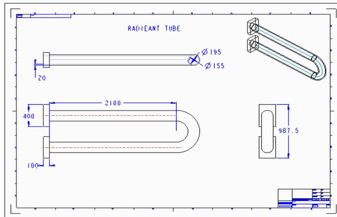
**FIG 1. 9 3D DETAILED DRAWING OF RADIANT TUBES**
