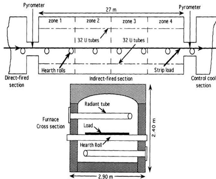
FIG 1.5 SCHEMATIC OF THE INDIRECT-FIRED SECTION OF THE INLAND STEEL ANNEALING FURNACE
