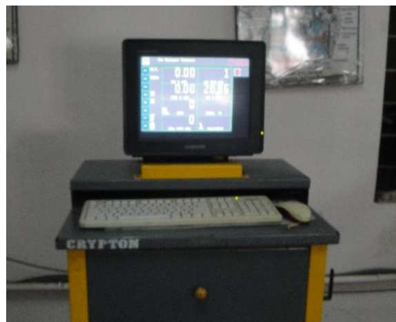
Fig. 4 Exhaust gas analyzer
