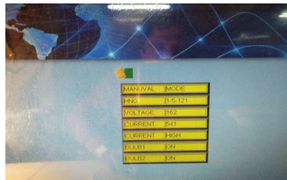
Fig (4.4) Parameters (Bulbs ON condition) are display on web server
