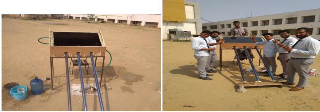
Figure2. Experimental Setup of Solar Still with Evacuated Tubes
