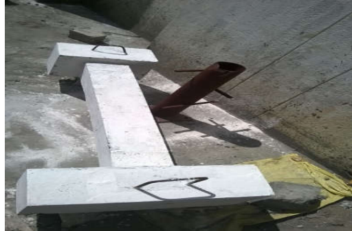
FIG:4 RC Column Specimen
