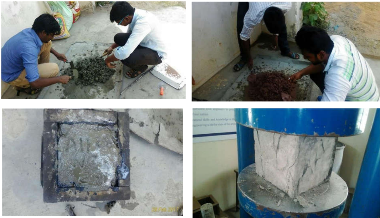
FIG.2 CASTING AND TESTING OF CONCRETE
