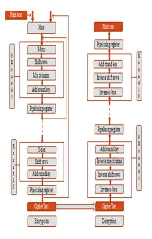
The decryption procedure is precisely the inverse of encryption procedure consisting conjointly four stages specifically InverseSubBytes, Inverse ShiftRows,InverseMixColumns, and AddRoundKey.
