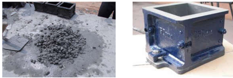
Fig.4 Mixing and Cube Mould
