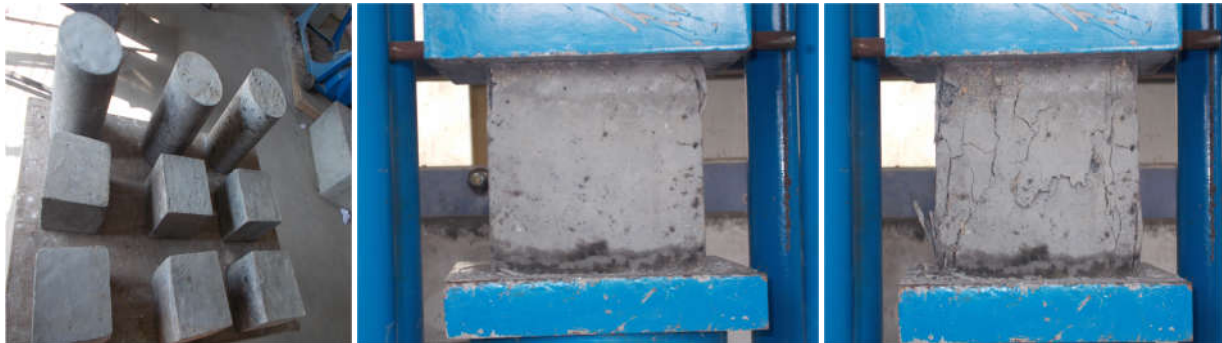
Fig.6 Testing of Cubes and Cylinders
