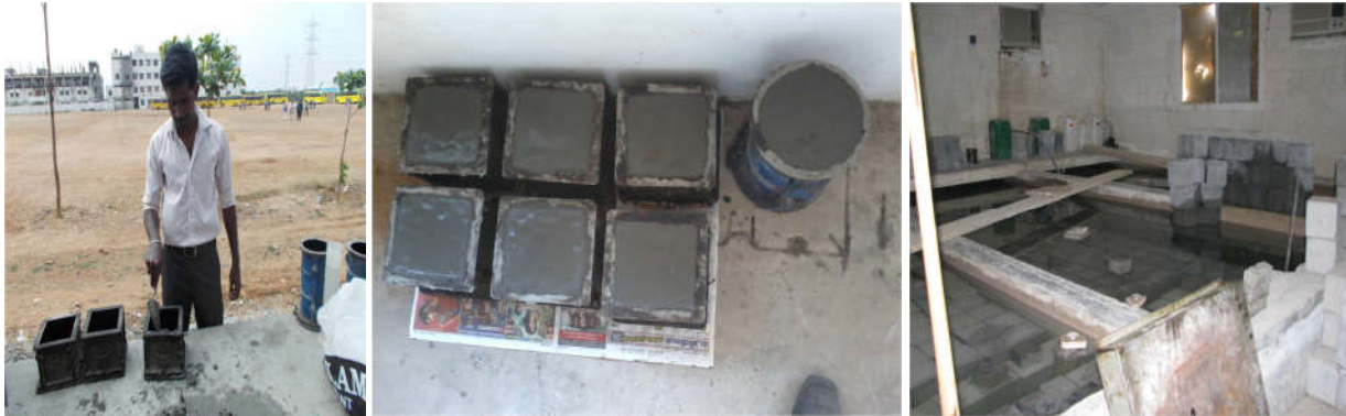
Fig.5 Casting and Curing
