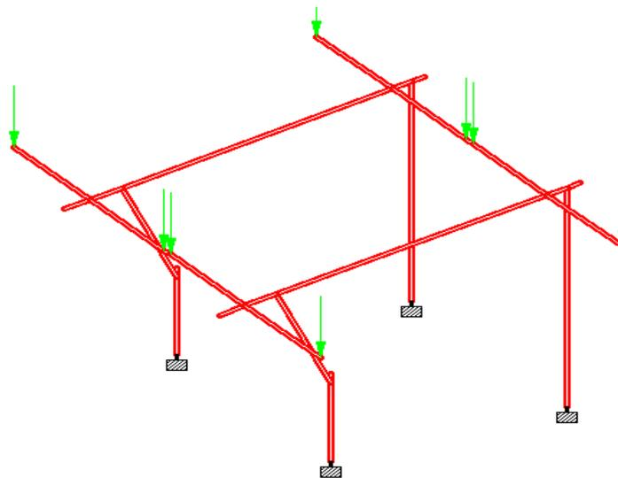
Figure 2 Staad.pro image of Solar Structure with nodal loads
